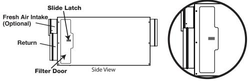
Step 2: Remove the filter by gently pulling it straight out of the unit. Insert new filter by gently pushing it straight into the unit. Make sure the AIR FLOW arrow on the filter is pointing into the unit.
