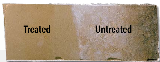
Drywall treated with Bora-Care with Mold-Care and placed in an incubator for 90 days.
