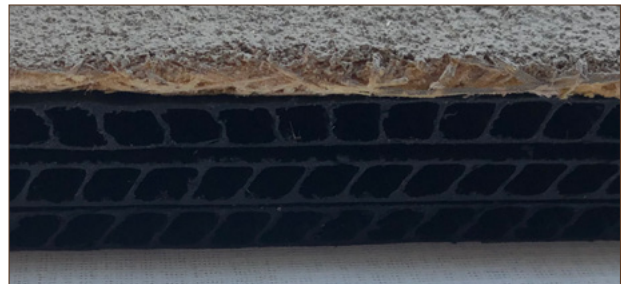
Example of Ventilation Strips
